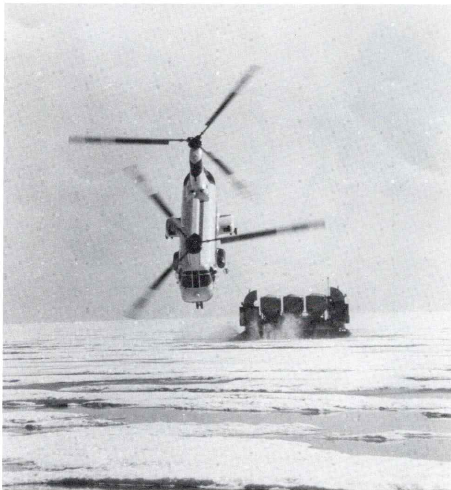
Tow ability of Columbia Helicopters' Boeing Vertol 107 was clearly demonstrated twice this year in dramatic tests, one done on Puget Sound and the other on Alaska's North Slope. The Vertol provides the power to tow the barge which is riding on a cushion of air. The nose attitude of the helicopter was as much as 35 degrees with the aircraft approximately 20-30 feet above the water.
