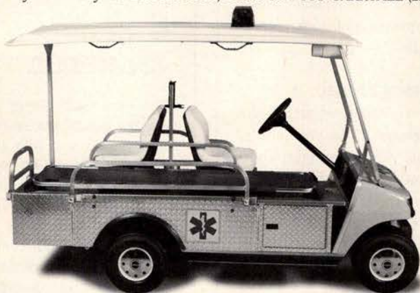
Tourall Ambulance with stretcher, storage space for medical equipment, single front seat and single back seat for attendant.
