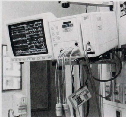
*The power columns in patient cubicles are equipped with monitors that display physiologic parameters such as blood pressure, heart rate, and respiratory measurements. The information collected about each patient is transmitted to the bedside computer workstation.*
