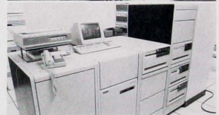
*(Top) PCs to be installed for the secretaries in the new building are lined up in front of two VAX 11/780 units already in operation. (Bottom) In the drawers of this hierarchical storage controller are disk drives containing disks on which information is stored. Disks can be removed and replaced, similar to floppy disks on a PC.*
